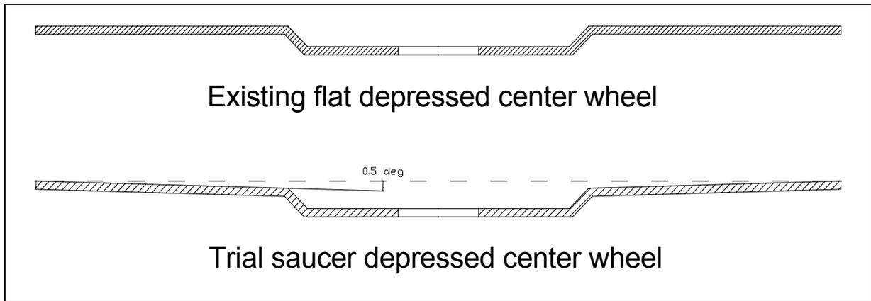
**Figure 11 – Modifications to Depressed Centre Wheel**
