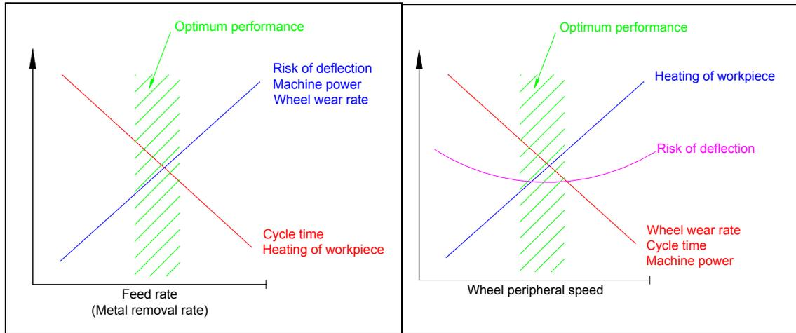
**Figure 5 – Machine operating parameters**
