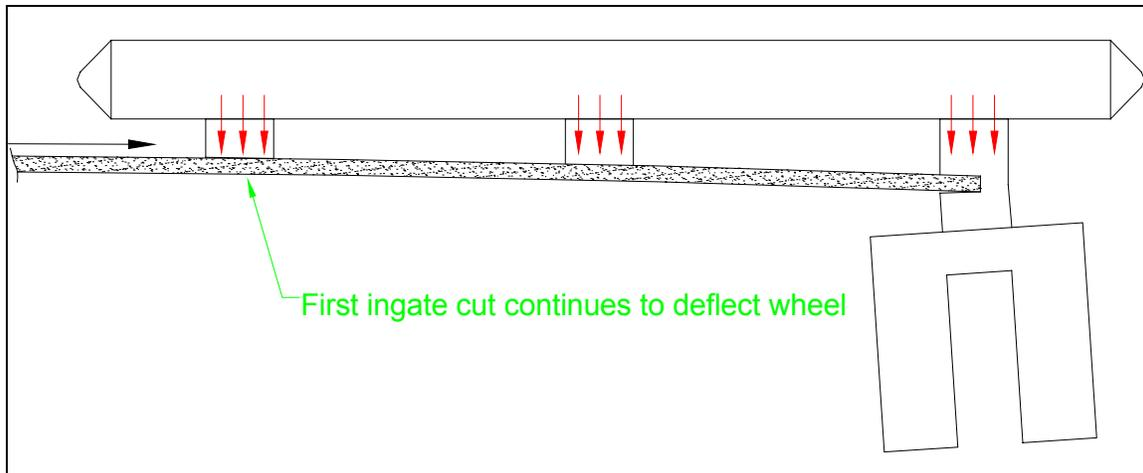
**Figure 8 – Forces on Wheel During Cutting (multiple ingate)**
