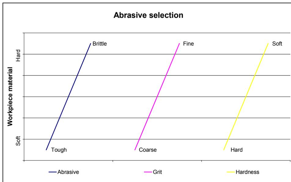
Figure 4 – Abrasive Wheel Selection
