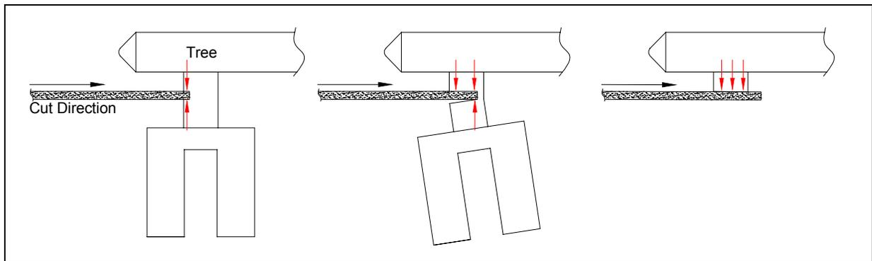
**Figure 7 – Forces on Wheel During Cutting (one ingate)**
