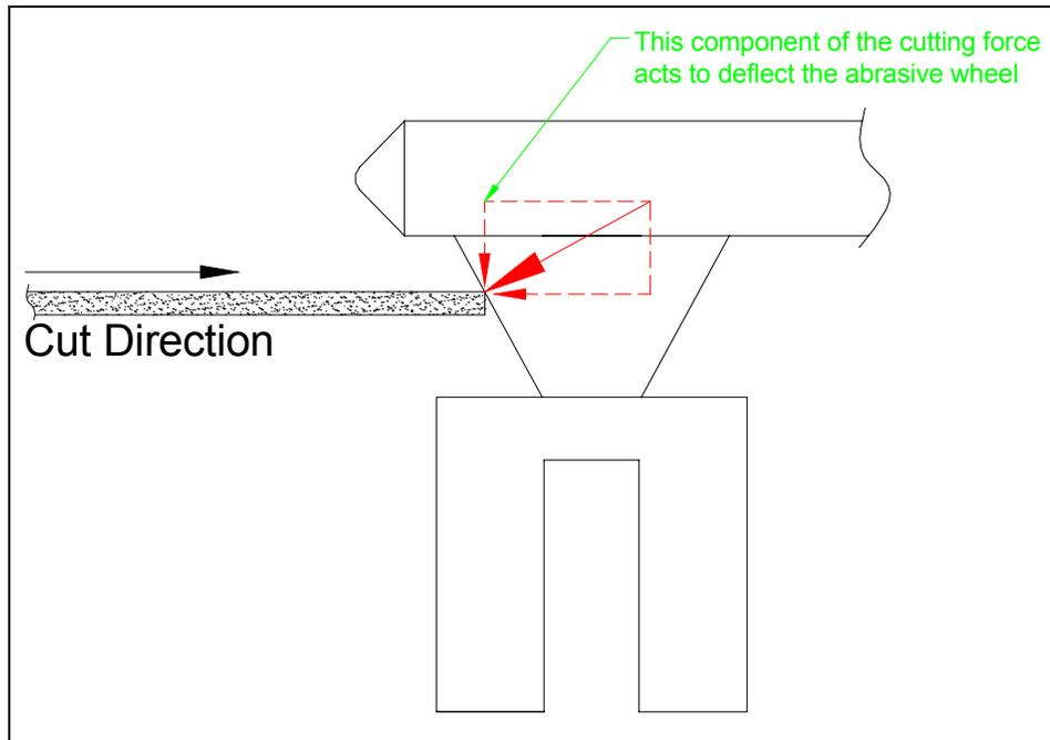
**Figure 9 – Cutting of Angled Ingates**
