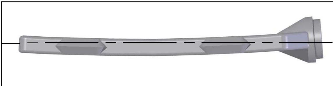
**Figure 1 – Example of bowing along the axis of wax sprue**
