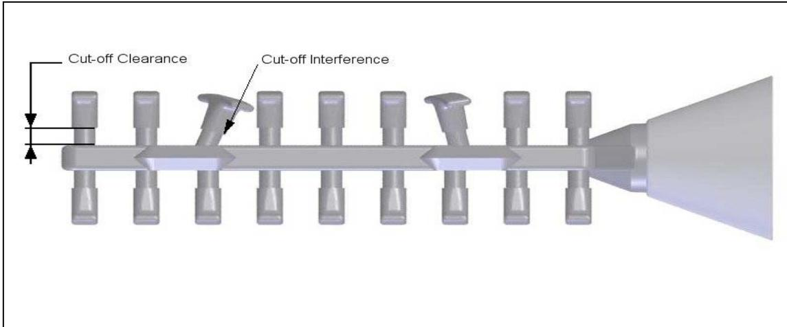
**Figure 2 – Interference in the cut off area**
