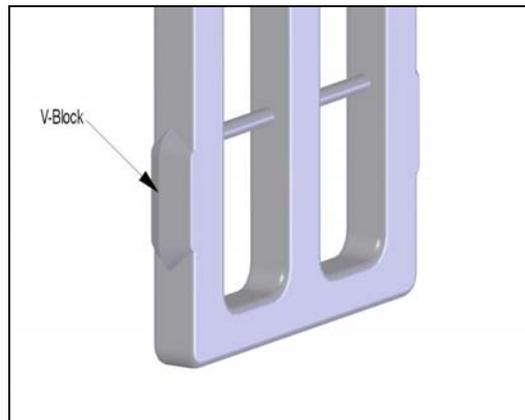
**Figure 3 – V Block along axis of sprue**
